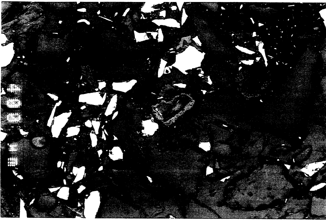
Figure 3. Geco tailings. The pyrrhotite grain at the centre of the photo is almost completely dissolved and rimmed by Fe hydroxide. Pyrite remains unaltered. Width of photo corresponds to 40 mm. Plane-polarized reflected light.
