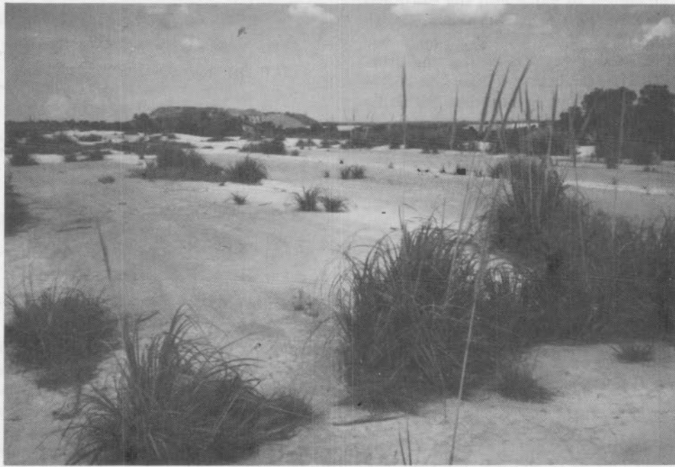
Fig. 5—Appearance of test panels of stabilized gold residue three years after laying
